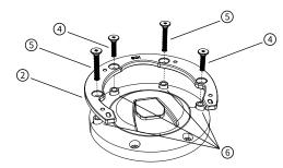
3. Place part 1 on top of part 2 (note to align the holes), put in the screws, and tighten the screws in turn. (Torque: 1.5N·m)
